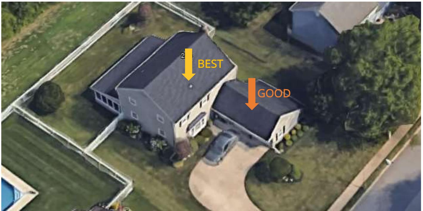
Based on our analysis, the best roof plane to install solar panels is the southeast-facing roof space on the front of your home. If you need more solar power, a second option is the southwest facing roof above your garage. This roof space will get some morning shading from the tree in front of your home and some shading from your main home in the afternoon, but can still be an effective space for solar panels.
